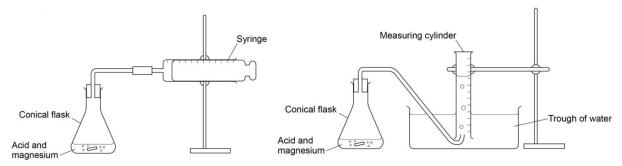
A gas syringe (left) or trough (right) should be used to measure a volume of gas. The **syringe** is more easily operated but has a greater uncertainty than the **trough**. The measuring cylinder must be completely **full of water** at before the beginning of the practical. The **meniscus** will fall
