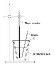
In an **enthalpy change** practical, the temperature change needs to be accurately measured. This is done by **minimising** heat loss or heat gain from the surroundings. A polystyrene cup and lid is used to **insulate** the reaction mixture from surroundings. The stirrer is used to ensure thermal energy is spread evenly in the reaction mixture. The bottom of the thermometer must be **in** the reaction mixture.
